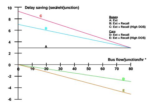
\* Bus flow/junction/hr = Number of buses given priority/intersection/hour Ext = Green extension Recall = Red truncation DOS = Degree of saturation
